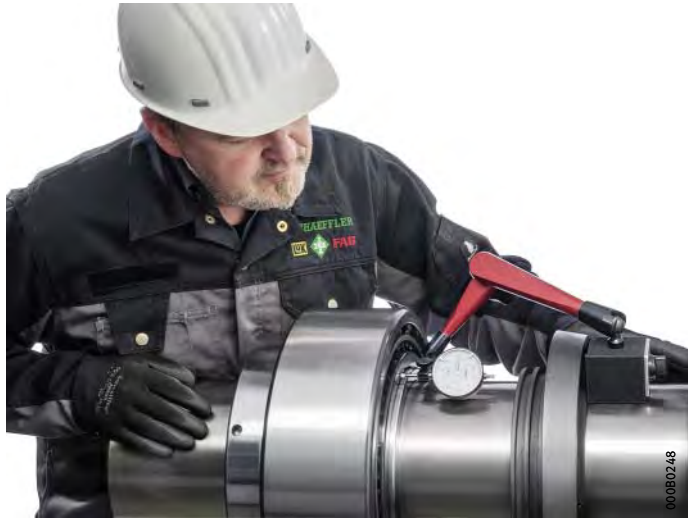
Figure 7 Mounting of toroidal roller bearing
