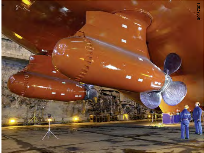
Figure 1 Compact drives with a 360° rotation facility fitted to the stern of a ship
